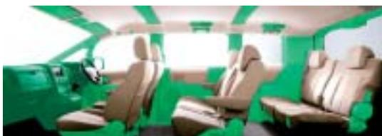
Many plastic fittings in the *Delica D:5* are made from easily recyclable thermoplastic resin (green areas)
